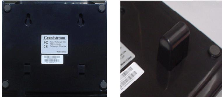
To position the phone on the wall, place two fixed hangers on the wall, hang the back of the phone on the fixed hangers. The two sustaining brackets will balance the bottom of the phone and position the phone on the wall.
