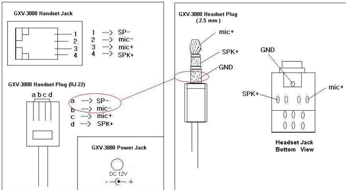
The left side of the diagram illustrates the RJ22 (handset plug) pin assignment; the right side illustrates the 2.5mm headset plug. Additional adaptors are necessary to connect the phone to an external speaker or intercom/paging system. (Adaptors can be purchased from an local electronics store).
