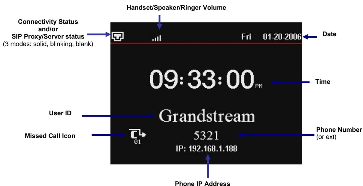
The LCD display disappears when the screensaver is on. If you do not want the LCD display, you can turn it off.
