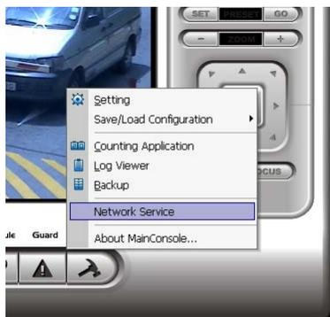
There are 3 types of network services: live streaming server, remote playback server, and 3GPP service. From the Main Console, go to Config > Network Service to obtain the Network Service panel.
