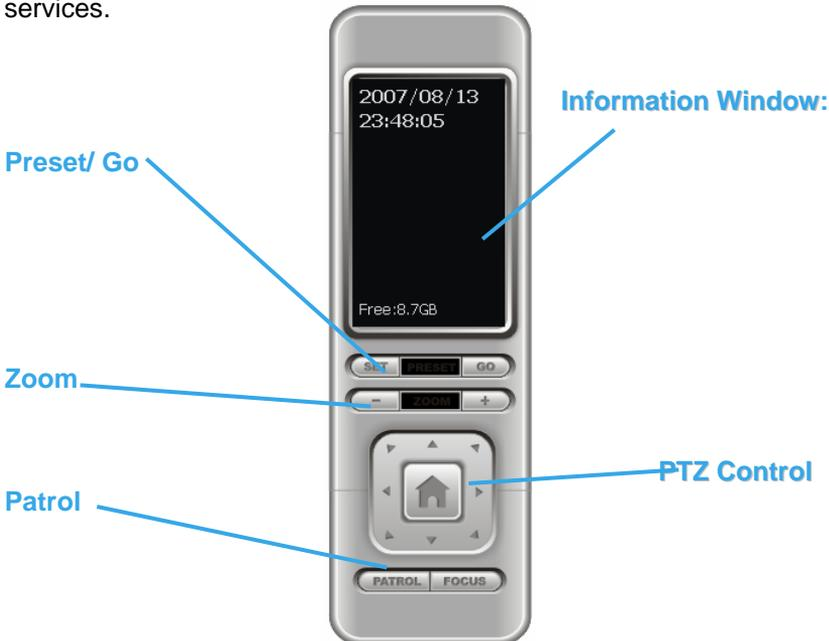
**Information Window:** Display date, time, free HD space, CPU temperature, fan speed, and customized text. To customize Information about window's setting, go to Config > General Setting > General
