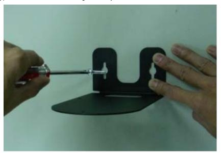
2. Fix the camera to L-type bracket with two supplied screws.
