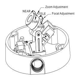
4. When the ICA-525 focus adjustment has been completed, use the provided L-wrench to fasten the tamper-resistant housing to the main body.
