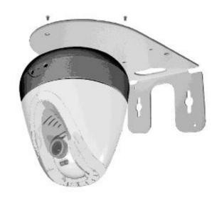
2. Fix the bracket and camera to the ceiling using two holly wall anchors and screws.
