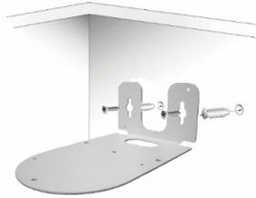
2. Fix the camera to L-type bracket with the two supplied screws.
